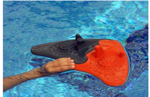
This fully functional 3D printed prototype was tested in real conditions and enabled AIJU to verify and validate the design fast.
